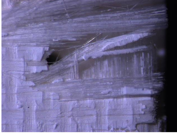
Figure A. 11: Fracture surface of specimen #3, tested in tension to failure at 1200°C in air
