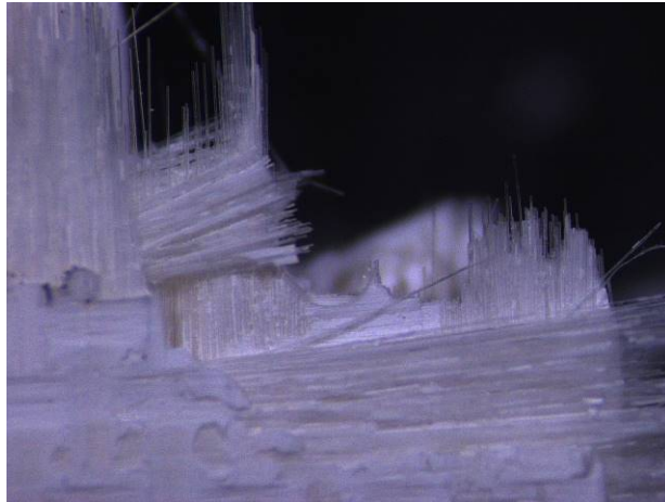
Figure A. 55: Fracture surface of specimen #9, tested in creep at 1200°C in steam ( \sigma_{cr} = 116 MPa, t_f = 0.61 h)
