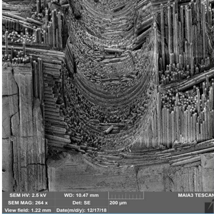
Figure 49: Fracture surface of an N720/A specimen with diamond-drilled holes tested in creep at 1200°C in air ( \sigma_{cr} = 93 MPa, t_f = 6.55 h)
