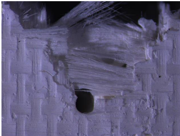
Figure A. 38: Fracture surface of specimen #12, tested in tension to failure following 100 h creep at 46 MPa at 1200°C in steam
