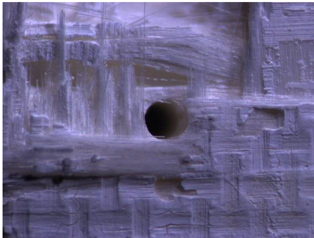
Figure A. 13: Fracture surface of specimen #3, tested in tension to failure at 1200°C in air
