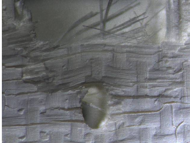
Figure A. 24: Fracture surface of specimen #6, tested in creep at 1200°C in air ( \sigma_{cr} = 69 MPa, t_f = 30.95 h)
