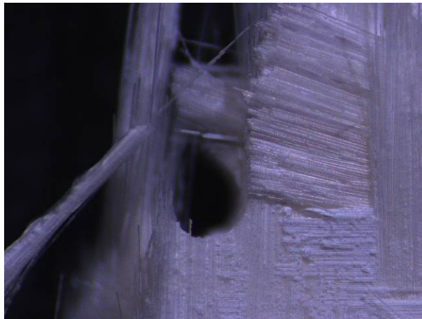
Figure A. 4: Fracture surface of specimen #3, tested in tension to failure at 1200°C in air
