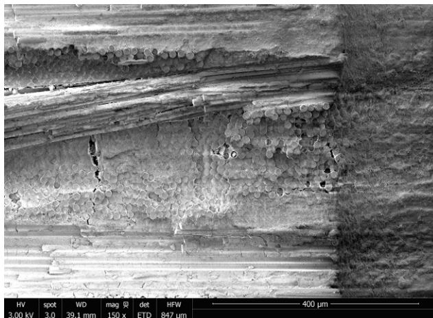
Figure C. 46: Fracture surface of specimen #10, tested in creep at 1200°C in steam ( \sigma_{cr} = 93 MPa, t_f = 6.05 h)
