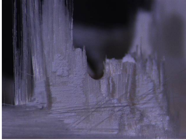
Figure A. 48: Fracture surface of specimen #9, tested in creep at 1200°C in steam ( \sigma_{cr} = 116 MPa, t_f = 0.61 h)
