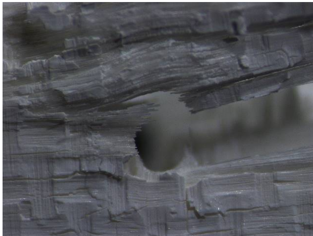
Figure A. 21: Fracture surface of specimen #7, tested in tension to failure following 100 h creep at 46 MPa at 1200°C in air
