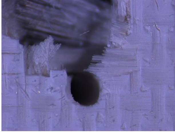
Figure A. 37: Fracture surface of specimen #12, tested in tension to failure following 100 h creep at 46 MPa at 1200°C in steam
