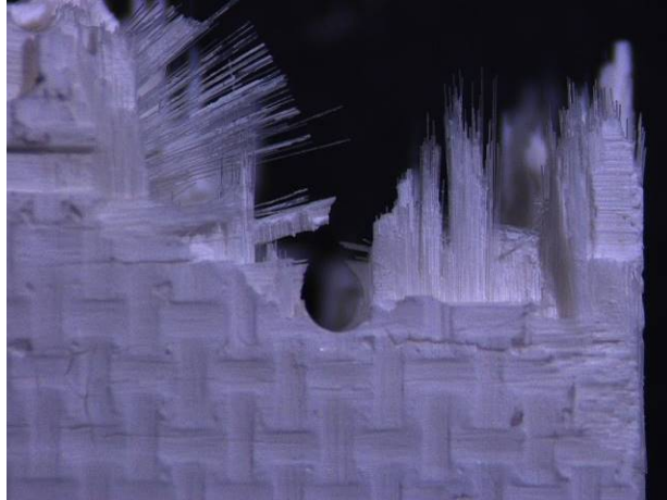
Figure A. 43: Fracture surface of specimen #12, tested in tension to failure following 100 h creep at 46 MPa at 1200°C in steam
