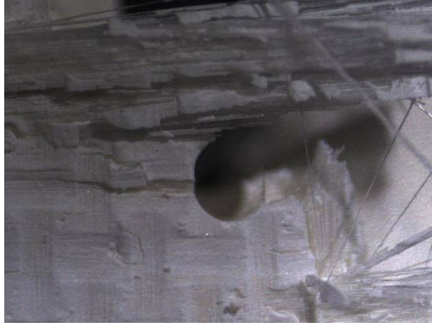
Figure A. 28: Fracture surface of specimen #4, tested in creep at 1200°C in air ( \sigma_{cr} = 118 MPa, t_f = 0.59 h)
