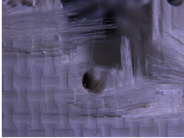
Figure A. 54: Fracture surface of specimen #9, tested in creep at 1200°C in steam ( \sigma_{cr} = 116 MPa, t_f = 0.61 h)
