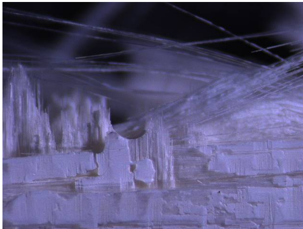
Figure A. 6: Fracture surface of specimen #3, tested in tension to failure at 1200°C in air
