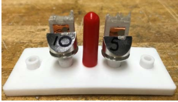
Figure 23: Coated specimen prepared for SEM examination
